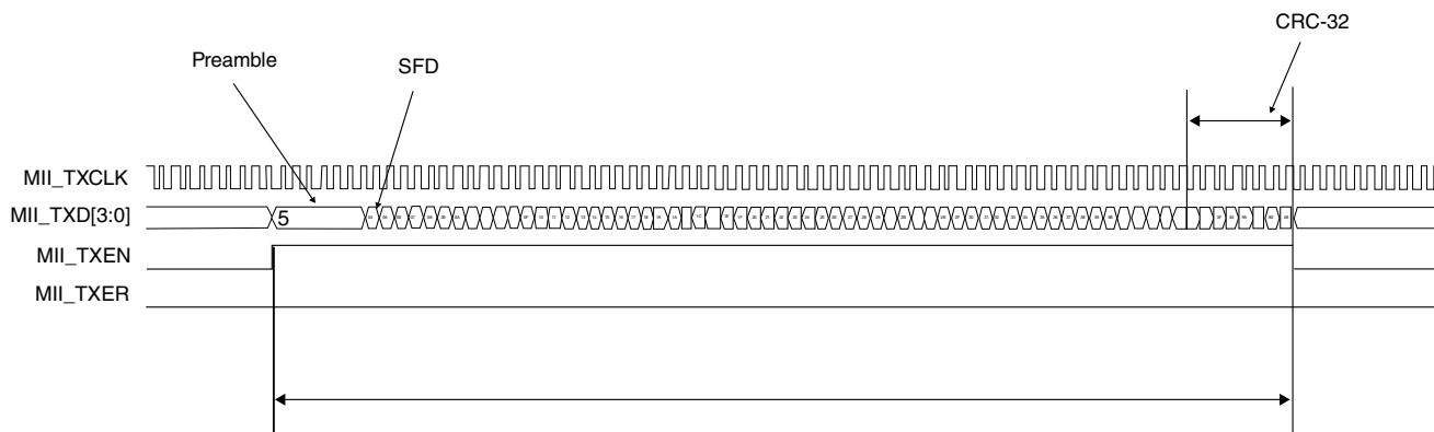
Figure 45-22. MII transmit operation
