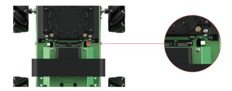
4 Connect the cable of 3D depth camera to No.2 port on Jetson Nano board.
