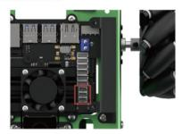
3 Connect USB cable of monocular camera to No.1 port of Jetson Nano board.
