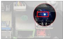
3 After robot boots up successfully, robot is default to AP direct connection mode and generates a WiFi starting with "HW". The initial WiFi password is "hiwonder".
