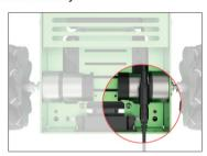
4 Red indicator means robot is being charged. It will turn green after robot is fully charged. It takes about 4 hours to fully charge the battery. Please unplug the charger in time once battery is fully charged to avoid overcharging.
